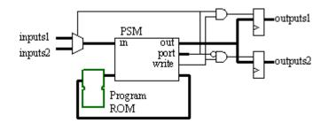
The diagram below shows how the use of two PSM macros simplifies the I/O interface. It may also help with the layout of a design in a large device. (After all, if you were implementing hardware state machines, they would be implemented separately.)
