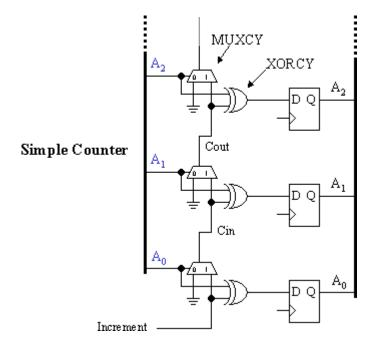
The carry logic is able to implement an increment function without using the look up table (LUT). The operation of each bit is defined by the following truth tables. Observe how the MUXCY propagates the carry signal.
