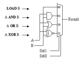
For each bit of the operands, we can see a 4-input function -- a perfect fit for a look-up table. In this way, the entire 8-bit logical group (including the multiplexer) can be realised in just 4 "slices" rather than 20 slices (4 "slices" for each AND, OR, and XOR, plus 8 for a 4:1 multiplexer). This reduction in size again provides the benefit of higher performance.
