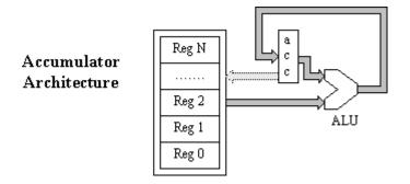
The **accumulator structure** is almost certainly associated with registers or memory to hold the various variables. The advantage of the accumulator structure is that one of the operands and the destination for the result is implied and does not need to be specified in the instruction encoding. Hence, the instruction encoding only needs to reserve bits to identify the remaining operand, and less logic is required to select the register or alternative source.
