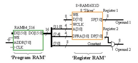
The program memory acts as the controller and is formed using block RAM. The variable data will be held in registers, and these are made cost-effective via the highly efficient distributed dual-port RAM. Without this distributed RAM option, the 44 CLBs (88 "slices") required to implement the register bank alone would already exceed the size of the complete PSM implementation!
