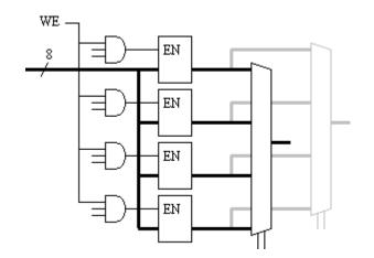
We must now add the operand selecting multiplexers and clock-enable gates to the registers. A 4-to-1 multiplexer would require a complete slice per bit by combining the two LUTs and the dedicated MUXF5. Hence the 8-bit multiplexer requires 8 slices.
