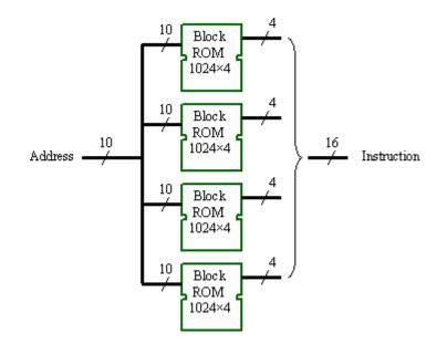
Increasing the size of the program memory sounds like an easy thing to do, but the PSM is now required to support the extended address range. To increase from 256 locations to 1204 requires that the program counter grow from 8 to 10 bits. Likewise, the width of the CALL/RETURN stack must grow. However, these only increase the size of the PSM by a few "slices". The real issue is determining how to specify the address operand in the JUMP and CALL instructions.
