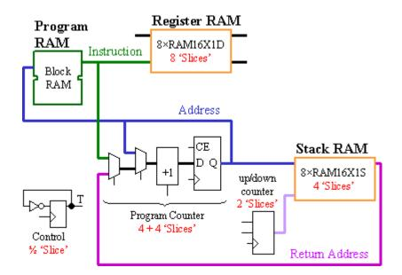
Distributed RAM has been used twice to provide a total of 256 bits of memory in 12 "slices". Using flip-flops and logic to replace these memory structures would require 152 "slices", which is more than double the size of the complete KCPSM (35 CLBs in Spartan-II provide 70 "slices"). Using block RAM to implement these small memories would be wasteful and would impact the flexibility of a PSM to be used multiple times in devices, especially small ones with limited block RAM.
