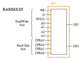
The 16 RAM cells provide all the functionality of a 1-bit, 16-register bank, complete with selective write enable. The second port enables a second operand to be accessed in the same way that a second multiplexer was used with discrete registers. With this great feature, an 8-bit, 16-register bank can be implemented in just 8 "slices" (compared to 88 "slices") and significantly increases performance.
