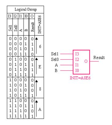
The above truth table derives the INIT value for each LUT forming the logical group. The same mapping should be achievable via synthesis tools now that we are breaking the description of the ALU down into manageable pieces.
