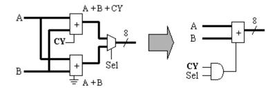
Rather than use the select signal as a multiplexer control, we now use it as a masking control to the CARRY (CY) signal. Since this is a single AND gate, it only costs a ½ "slice" compared with 4 "slices" for a multiplexer and a further 4 "slices" for a second adder. Although this is a simple observation, you must consider this when writing any HDL code.
