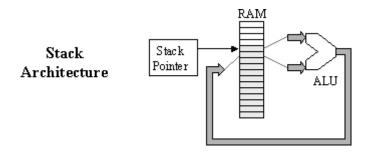
The **stack architecture** is probably the most efficient in terms of silicon resources, as it links directly to memory that is forming the stack and requires no data selection logic other than the stack pointer. The instruction encoding is also very efficient because the location of both operands and the result are implied as being the top of the stack.
