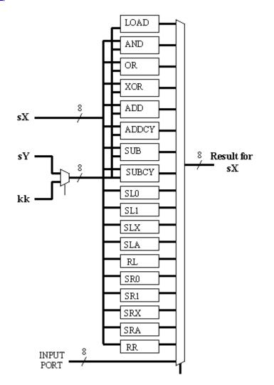
The apparent requirement for a 19-input multiplexer is alarming! Even with the dedicated multiplexers within the logic slices (MUXF5 etc), the size of this multiplexer for the 8-bit data width would be 48 "slices". This is very expensive, considering that each actual ALU function has yet to be implemented. This multiplexer would also require 5 select lines -- it would be an interesting task to encode these from the 4 primary bits and various "spare bits" of the instruction words.
