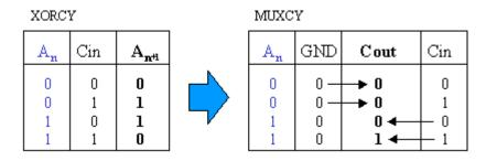
Because each logic "slice" contains the carry logic components and flip-flops for 2-bits, the required 8-bit program counter to access 256 memory locations can be implemented in just four "slices". However, the program counter must do more than increment.
