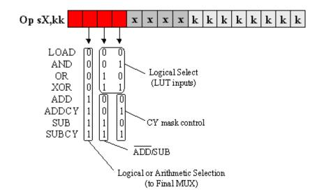
The ALU also generates flags used in some operations (i.e., ADDCY) and program flow control. KCPSM has a CARRY flag and a ZERO flag, but you may decide that other flags are more useful in your own PSM processors. Each flag may be implemented using a simple clock enable flip-flop to ensure that they are only updated during appropriate ALU operations.
