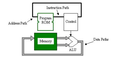
Given that there is no real restriction on the number of virtual pins the PSM can have, it is possible to explore all of the aspect ratios supported by the block RAM. At first, it may appear reasonable to adopt 8-bit instructions to be the same as the data path. This would make sense in a shared memory and bus system, but here we do not need to be constrained in that way.
