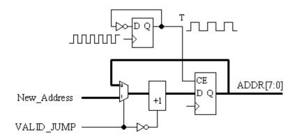
The toggle flip-flop is essentially the only logic forming the "state machine" of the PSM. The counter logic exploits the capability of the four "slices" very well.
