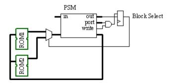
The multiplexer in the above diagram could be saved by using the block RAMs in 512×8 aspect ratio, then using the select bit to address the MSB (9th) address bit. However, the instructions will then be split across the RAM blocks, and programming the ROMs will become more challenging!
