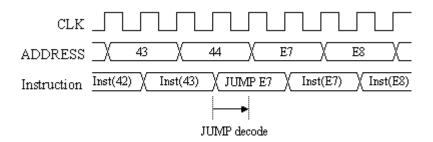
In the above timing diagram you can see that most instructions result in the simple increment operation of the program counter. When the JUMP instruction located at address 44 is read from the block ROM, the program counter is loaded with the new address value supplied (E7) and the address jumps on the next clock edge.
